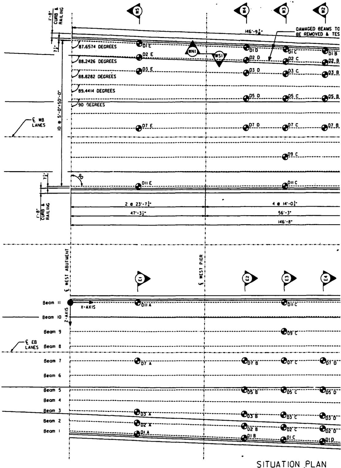
Figure 3.4. I-680 over County Road L34: Plan View of Beams and Deflection Transducer Layout.
